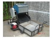
The harvested ginger roots are washed with water immediately after harvesting. Washing is done mechanically [batch] and rinsed several times with clean water.
