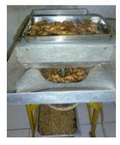
The clean ginger roots are sliced into a slab with a thickness of 3 to 4 mm. Slicing is done mechanically with a rotating knife, without adding water.
