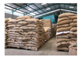
Coffee beans on the basis of size are packed in labeled production burlap sack [@ 60 - 90 kg] and stored in a clean and well-ventilated warehouse. Piles of sacks are propped on wooden pallets and do not lean to the wall of the warehouse.
