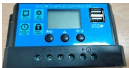
Gambar 4. Solar Charger Controller
