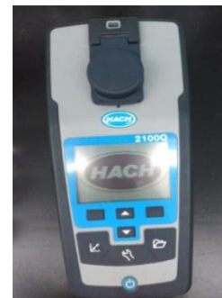
Gambar 9. Turbidity Meter HACH 2100Q
